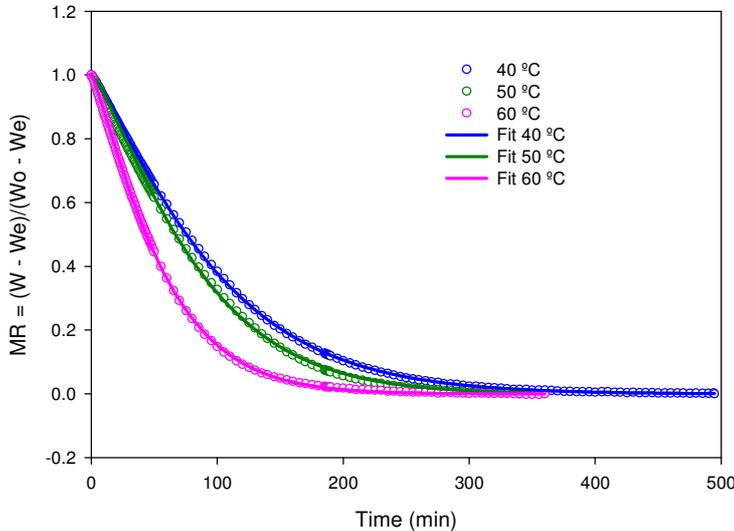
FIGURE 5: Fitting the moisture ratio with de Modified Page model at different temperatures and air velocity of 0.7 m/s.
