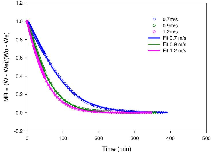
FIGURE 6: Fitting the moisture ratio with de Modified Page model at different air velocities and temperature of 60 °C.
