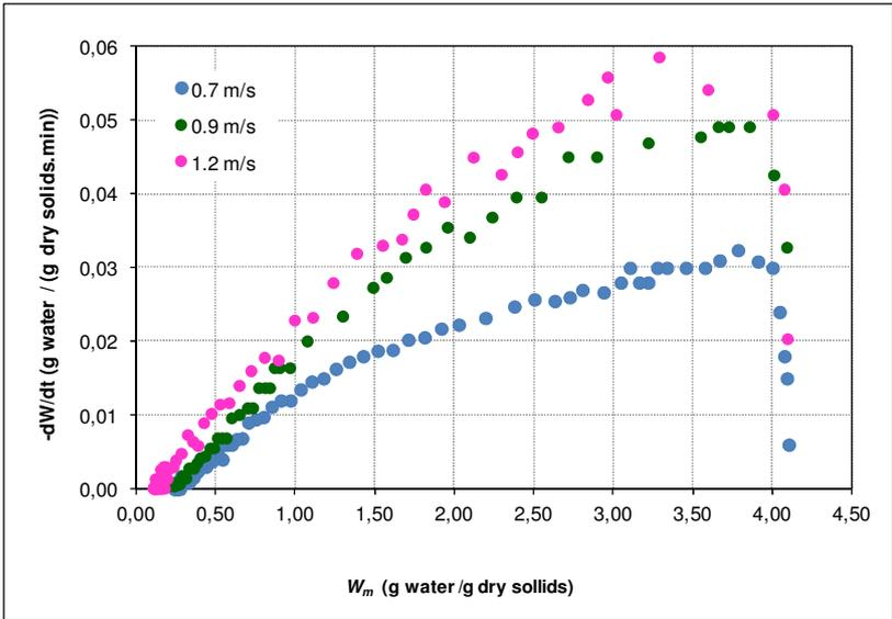
FIGURE 4: Drying rate curve versus moisture content at 60 °C and air velocity of 0.7 m/s, 0.9 m/s and 1.2 m/s.
