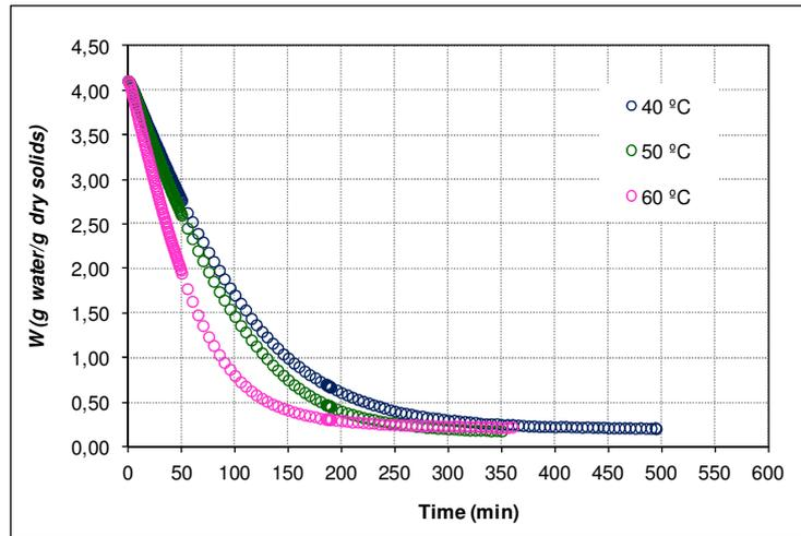
FIGURE 1: Profiles of moisture for temperatures of 40, 50 and 60 °C and air velocity of 0.9m/s.
