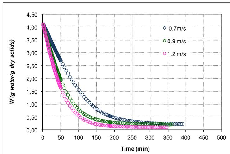
FIGURE 2: Variation of moisture along drying time for different air velocities at 60 °C.
