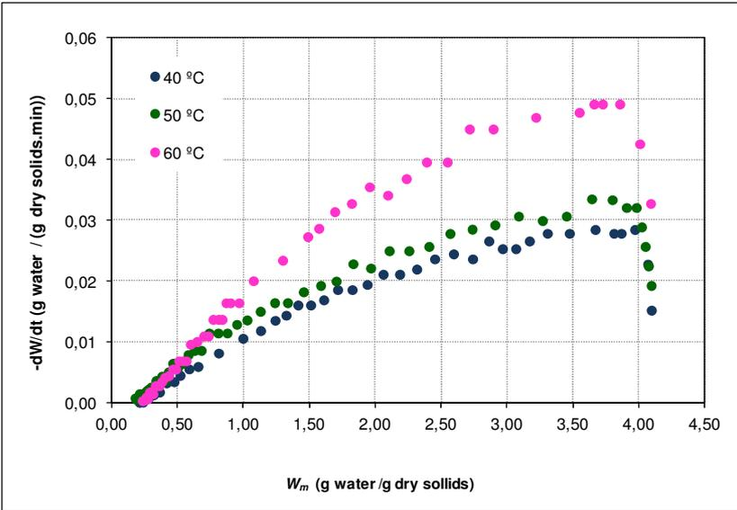
FIGURE 3: Drying rate curve versus moisture content for temperatures of 40 °C, 50 °C and 60 °C and air velocity of 0.9 m/s.
