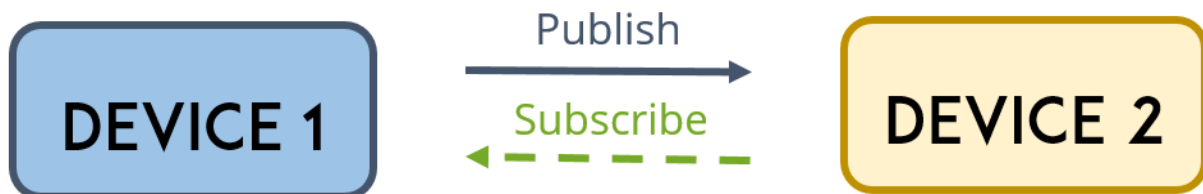
Figura 18 - Publicar/Assinar Mqtt [Fonte : randomnerdtutorials.com/what-is-mqtt-and-how-it-works/ ]
