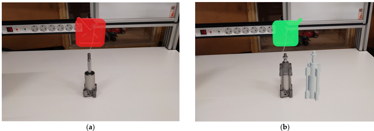
Figure 8. Validation process of the assembly quality control: (a) NOT OK; (b) OK.
