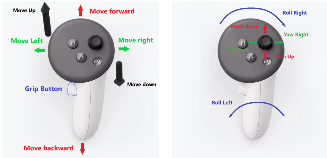
(a) Translational mapping and clutch (grip) input. (b) Rotational mapping: roll from controller orientation, pitch/yaw via joystick.
