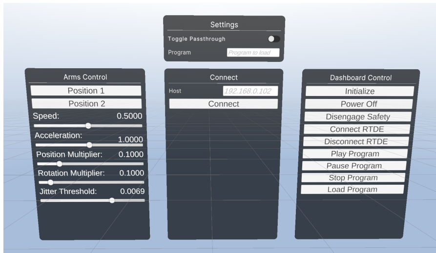
Figure 4.5: MR user interface panels for robot control.
