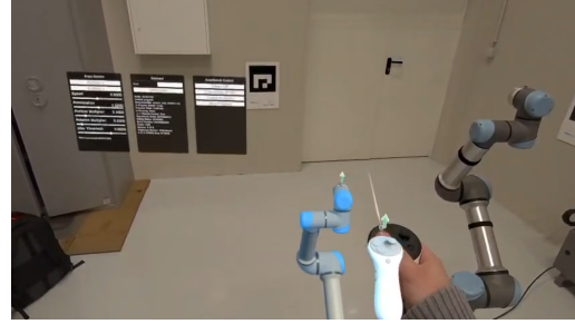
(b) Controller translation upward (TCP follows).
