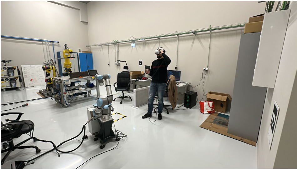
Figure 4.1: Development and debugging setup used during implementation, showing the UR5e, development workstation, and the HMD.
