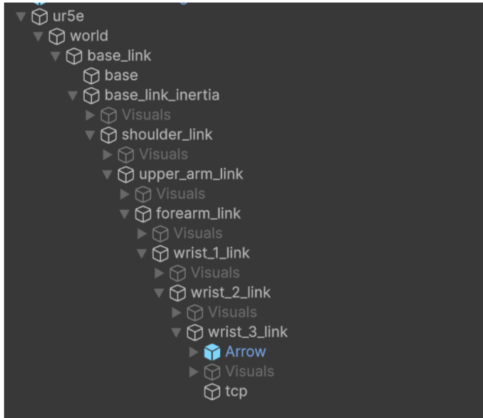
Figure 4.3: Unity hierarchy of the UR5e digital twin, showing the kinematic chain from base_link to wrist_3_link .
