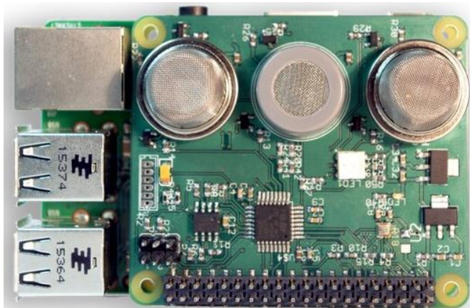
Figura 2-9: Altitude Technology Sensly HAT (Adaptado de (Altitude Tech, 2019)).
