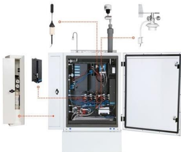
Figura 2-4: Aeroqual AQM65 (Adaptado de (Aeroqual, 2019)).
