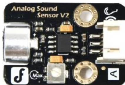
Figura 3-7: Sensor DFR0034 (Adaptado de (DFRobot Analog Sound Sensor, 2019)).
