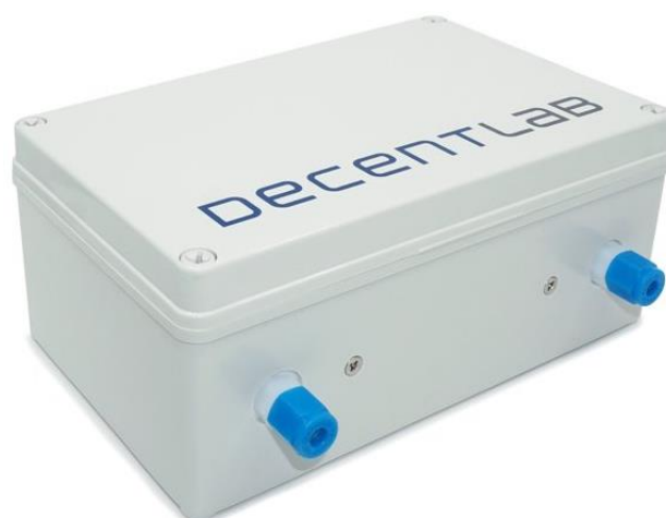
Figura 2-6: DecentLab Air Quality Station (Retirado de (DecentLab - Air Quality Station, 2019)).
