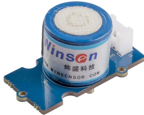
Figura 3-6: Sensor ME2-O2-Φ20 (Retirado de (Grove Oxygen Sensor, 2019)).
