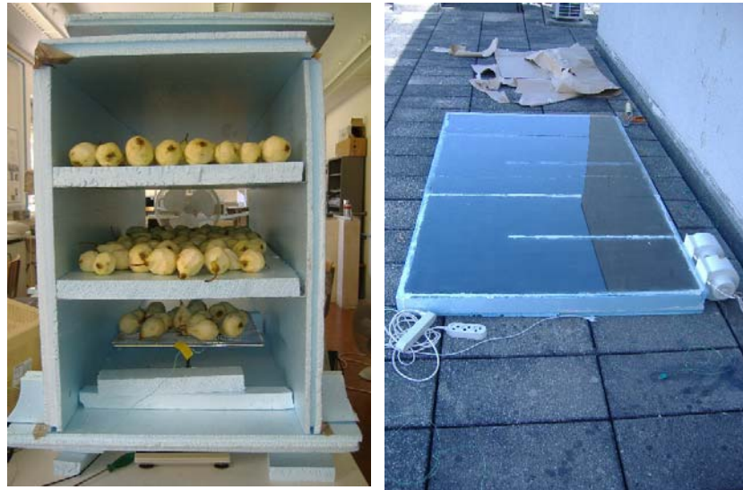
Figure 3. Drying tunnel and solar collector (UC).
