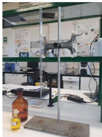
Figure 17. Titration of chlorine: (a) Reagents for titration; (b) Titration system
