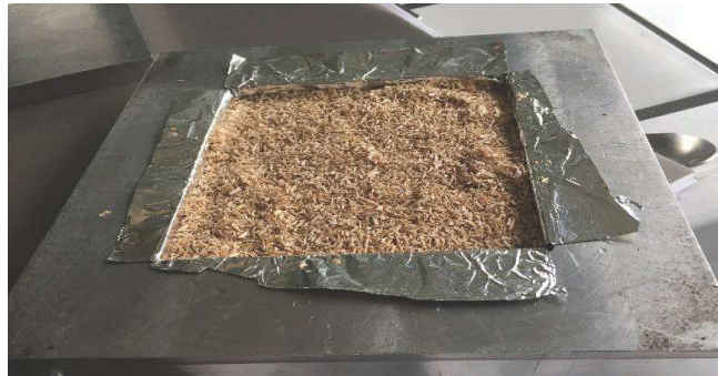
Figure 2. Stainless steel mold with ready-to-press mixture.
