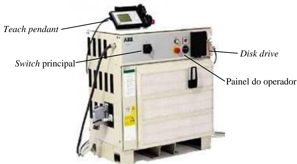
Figura 3-11: Controlador S4C com consola Teachpendant [24].
