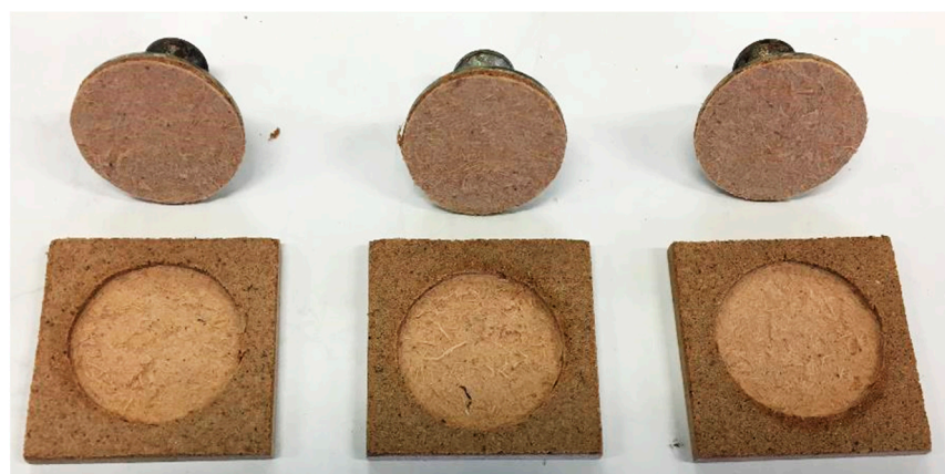
Figure 5. Photographic image of coated samples after adhesion testing, for the formulation with a 1:10 cork:resin mass ratio. The HDF substrate is visible in the circular areas where the coating was pulled off.
