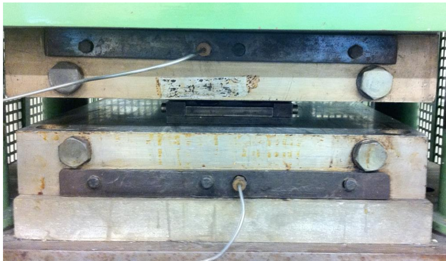
Figure 26 - Hot plated press (detail of how the moulds were pressured)
