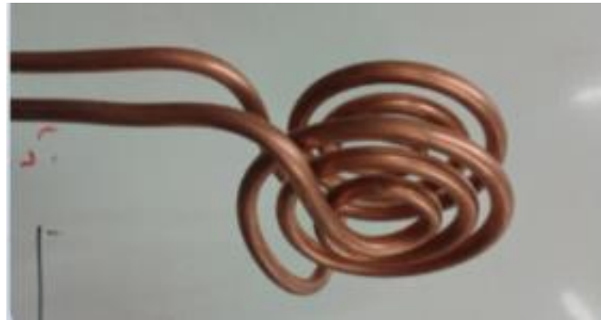
Figure 31 - Artisanal electromagnetic induction coil
