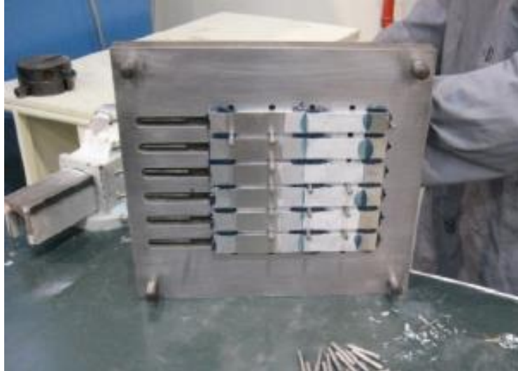
Figure 27 - Mould pin removal
