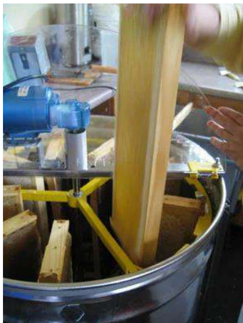
Fig 2: Put the uncapped frames into the honey extractor
