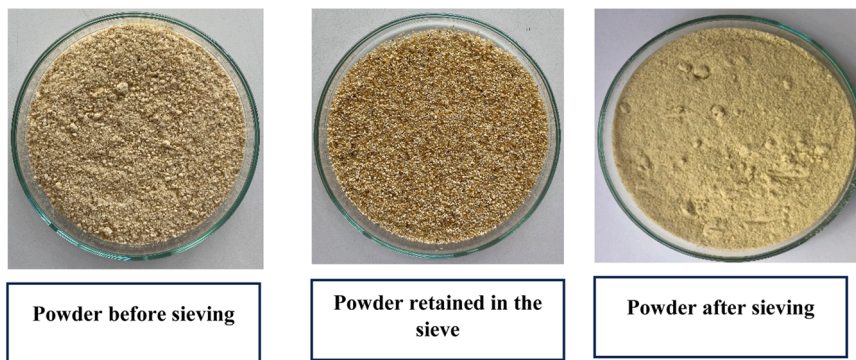
Fig. 11. Appearance of the powder produced by the extraction method of frozen DB on a cold surface (D1) before and after sieving.
