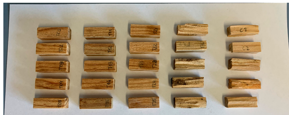
Figure 7. Wood samples after the 8-week exposure to termites. From left to right: 10% CA, 5% CA, 15% CA, untreated, and control.
