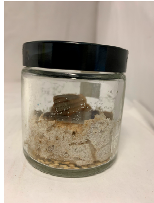
Figure 1. Termite durability tests according to EN 118:2013 [28].
