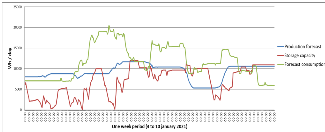
Figure 23 Comparison between the production forecast, storage capacity and consumption forecast in scenario C.
