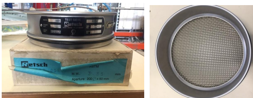
Image 20: Sieve used for the evaluation of fine dust content and mechanical durability (3.35 mm).
