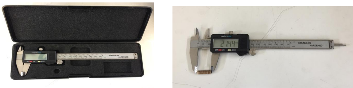
Image 14 : Digital caliper (right in its original box and left in measuring the length of a unit of pellets).
