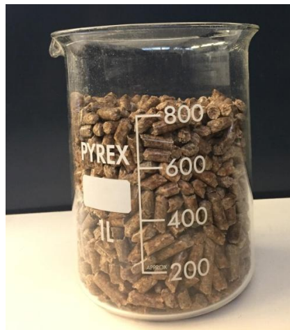
Image 19: Cup containing pine pellets used for the determination of bulk density ( V = 0.0008 m 3 ).
