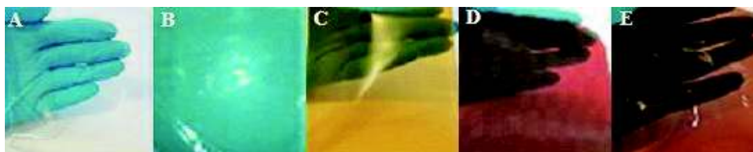
Fig. 5. Films of A) chitosan, B) chitosan cross-linked with genipin, and chitosan cross-linked with genipin and grafted with C) phenolic acids (Ch-PhAc-Ge), D) anthocyanins (Ch-Ant-Ge), and E) total phenolic compounds (Ch-TPhC-Ge) obtained from red wine.
