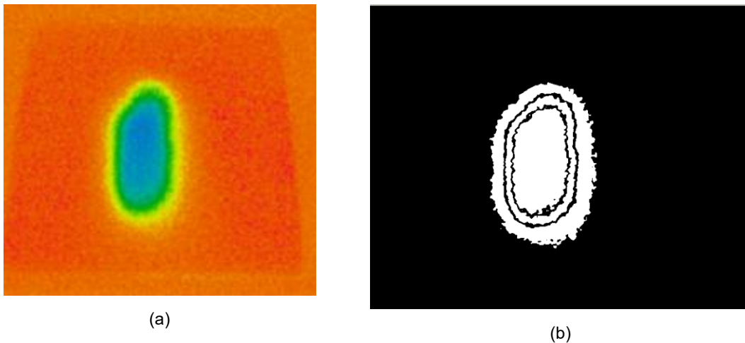
Figure 51- Visual comparison illustrating anomaly detection: (a) original thermal image and (b) image processed with the detect colors function.
