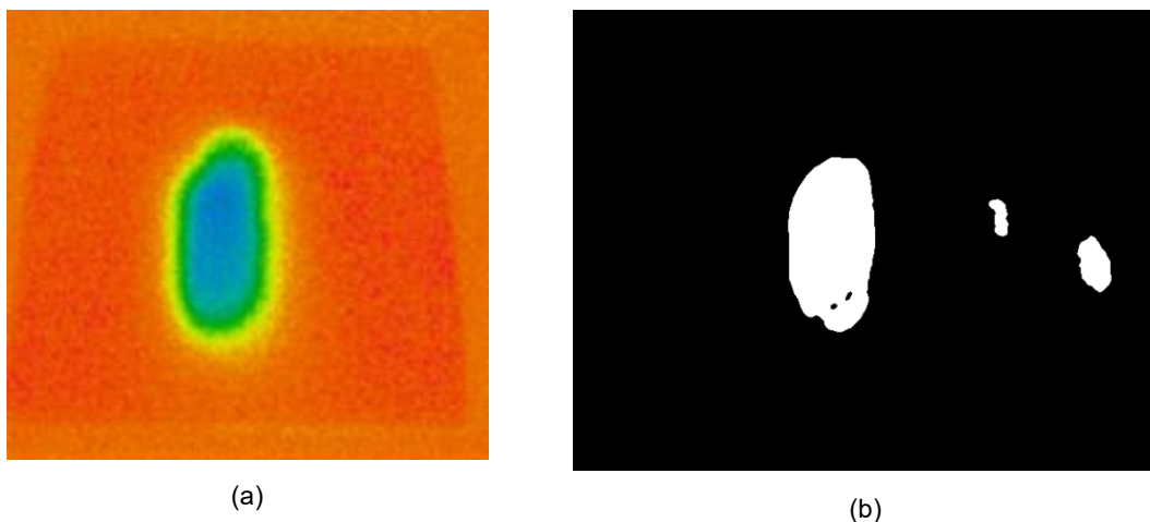
Figure 50- Visual comparison illustrating anomaly detection: (a) original thermal image and (b) image processed with the detect anomalies function.
