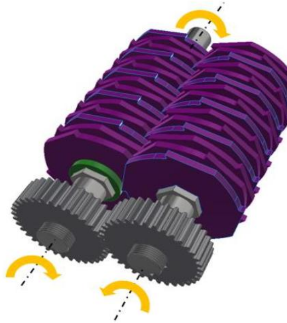
Figure 7. Arrangement of knives and transmission shafts.
